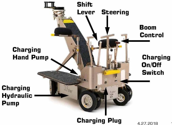
The electrical plug and switch are located on the back side below where the shift, steer and boom controls are located.
