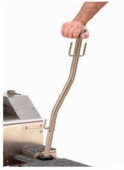
The push post will be used as a handle to operate the pump. Push and pull the handle to charge the hydraulic system.
